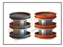
Sledge Hammer Cementing plugs are manufactured of graded rubber that is fused upon Aluminum core. This top plug can be used when dual plug system is not required and Bottom cementing plug can use when dual plug system is required. These plugs are completely PDC drillable.
